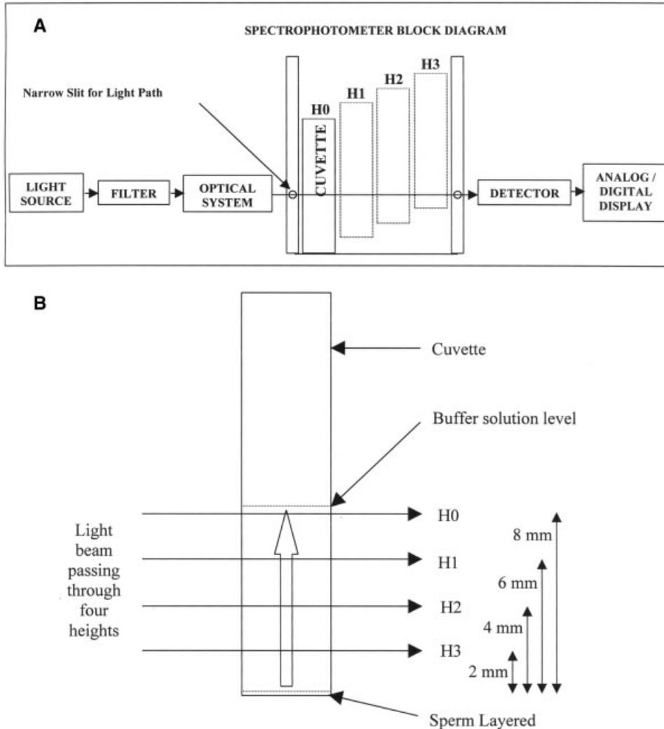
FIG. 4. A: Schematic block diagram showing the spectrophotometric system with the positions of the cuvette on vertical movement. B: Schematic diagram of the cuvette describing the buffer solution level, position of the sperm layer in the cuvette and the heights at which the cuvette is exposed to the spectrophotometric light beam.
