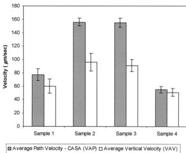
FIG. 6. Corresponding sperm velocity results of the same samples from CASA (Average Path Velocity) and New System (Average Vertical Velocity) displayed side by side. Result showing Mean  $\pm$  SEM of three experiments.
