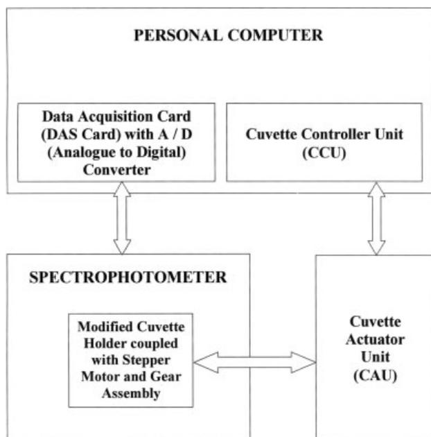
FIG. 2. Block diagram of the entire assembly for the spectrophotometer with static cuvette holders.
