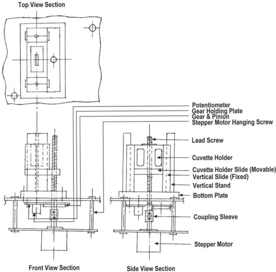
FIG. 1. Schematic diagram of the modified cuvette-holder along with stepper motor for the spectrophotometer with static cuvette holders.
