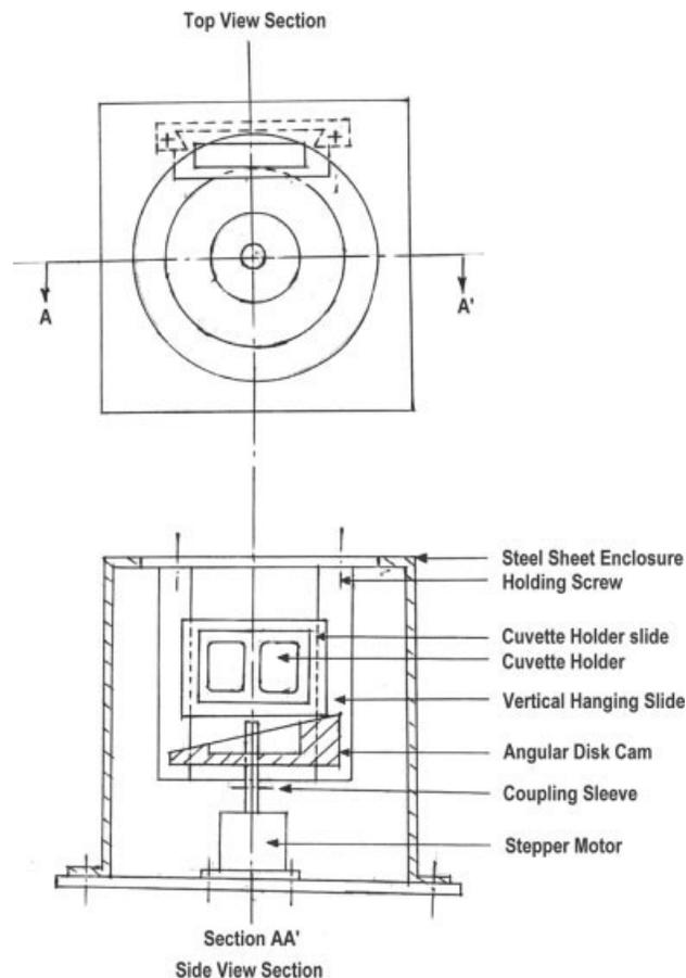
FIG. 3. Schematic diagram of the modified cuvette-holder along with modified cuvette-load arrangements for the spectrophotometer with circular moving cuvette holders.
